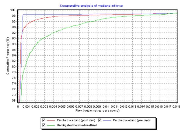
Figure 5: Cumulative frequency plot of discharge to perched wetland
