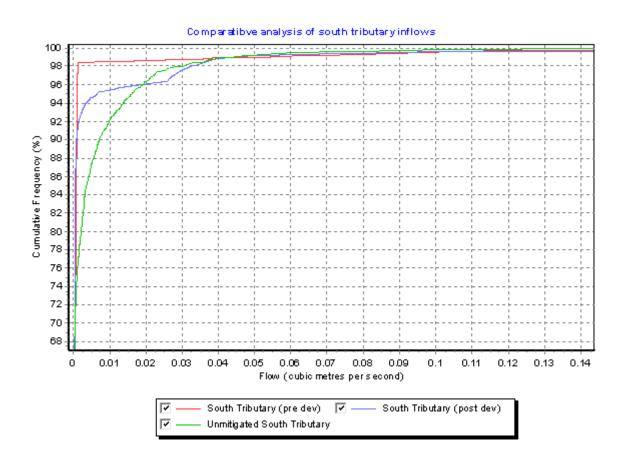
Figure 6: Cumulative frequency plot of discharge to Tributary 2
