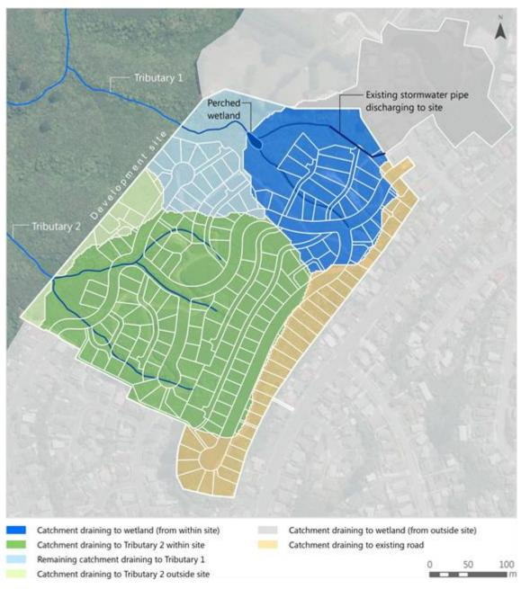
Figure 1: Pre-development catchments and drainage patterns
